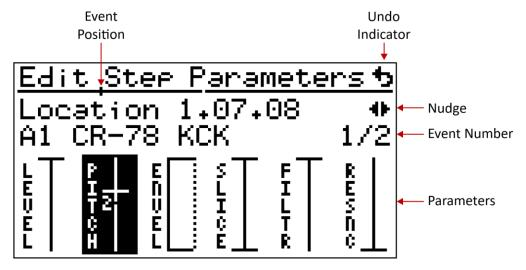
The exact location of the step is shown in bars + sixteenths + ticks. There are 24 ticks per sixteenth note. Location is also indicated on the horizontal bar. When playing, the play position is also shown on the bar.
