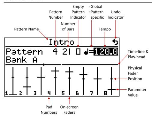
Pattern mode is the base mode of the machine. It is the mode in which patterns are recorded, modified, and played back. The screen shot above is annotated to point out the various bits of information on the screen in pattern mode.
