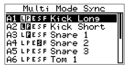
The screen displays the Multi Mode Sync settings for every track. This is the same setting that is on each of the individual fader mode setting menus (Shift+A), but conveniently all in one place.
