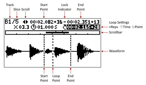
The exact start, end, and loop points are shown in minutes:seconds.milliseconds+samples format.
