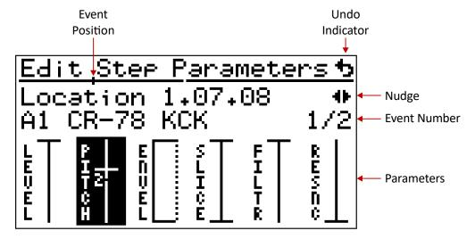
The exact location of the step is shown in bars + sixteenths + ticks. There are 24 ticks per sixteenth note. Location is also indicated on the horizontal bar. When playing, the play position is also shown on the bar.
