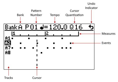
Step Program mode is an alternative method of creating and editing patterns. The screen displays a pattern in a DAW-like grid. The tracks are listed down the left side, and time across the top. The measure number is indicated in a time line at the top. Up to eight tracks are visible at a time. If more than eight tracks are present in the pattern, changing the bank will scroll the display vertically to show that bank's tracks.
