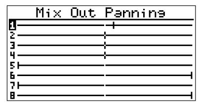
The pan screen controls how the outputs are mixed into the Mix Out jacks. Some planning is necessary when using stereo samples to ensure that the track's channels are properly panned, and that no mono samples play on those outputs.
